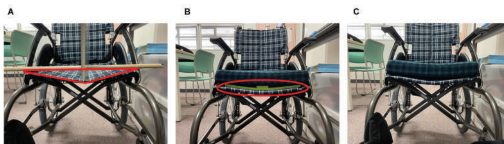
Figure 1. Measuring and padding wheelchair seat deflection. (A) Measurement of wheelchair seat deflection. Wheelchair (B) with deflection compensation pad and (C) without deflection compensation pad.
